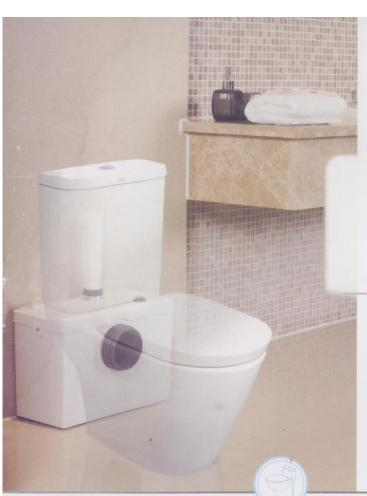
The ME90113 allows you to install an extra toilet almost anywhere in a home or office. It is economical and simple to fit, quiet in operation and (should it be necessary) can be serviced with ease. With a pumping performance of up to 9m in height or 90m in length, the ME90113 gives you unequalled performance and total flexibility of installation. Using standard I-inch (32mm) solvent weld plastic pipe allows you to install the unit almost anywhere.
