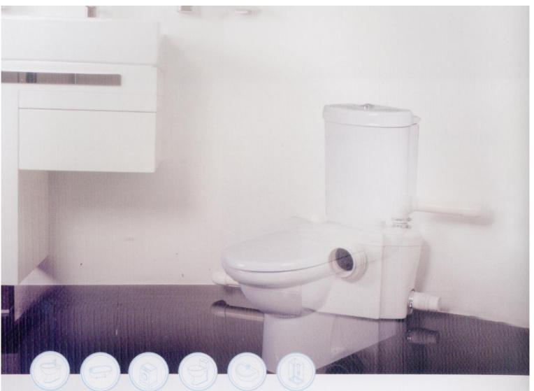
The ME90101 is simply a tank which is gravity fed from your toilet, washing machine, shower etc. with a built in pressure switch which detects the incoming waste and starts a pump combined with cutting blades. This reduces the effluent to an easy to pump fluid which is then pumped along small diameter pipes into the drains. A non return valve is fitted as standard so enabling the unit to pump up to 7m vertically.
